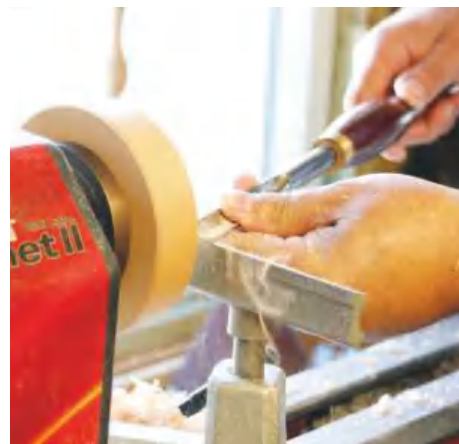
▲ Working the insides of bowls is easier with the tailstock removed
